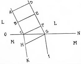
a physical Ray, or ABC and DEF to be two mathematical Rays, trajected from a very remote point of a luminous body through
